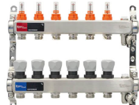
DISTRIBUTOR INCALZIRE PARDOSEALA, 1", 11 CAI, CU DEBITMETRE, AERISITOR MANUAL, ERMETIQ
