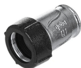
RACORD RAPID, FONTA ZINCATA, 1", FE, FILET EXTERIOR, GEBO
